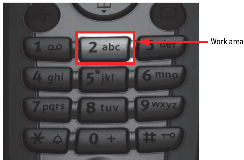
Figure 74: Example of autofunction AOI ( Show work area is on)
